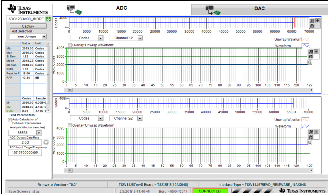
189. Idle-Channel Noise (No Input) for 2.5-GSPS, Dual-Channel Oscilloscope
