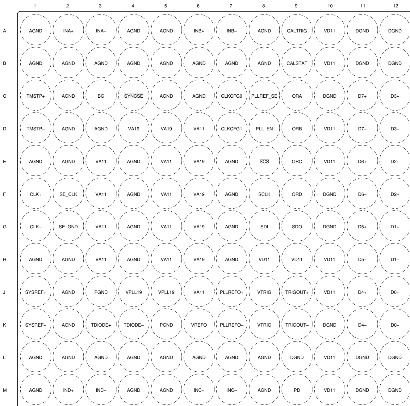
図 4-1. Quad Channel ALR Package, 144-Ball Flip Chip BGA (Top View)
