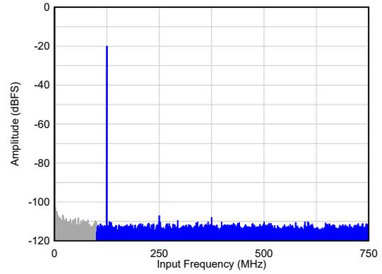
$F_{IN} = 125\text{MHz}$ ,  $A_{IN} = -20\text{dBFS}$ ,  $\text{SNR}_{\text{flat}} = 75.5\text{dBFS}$
