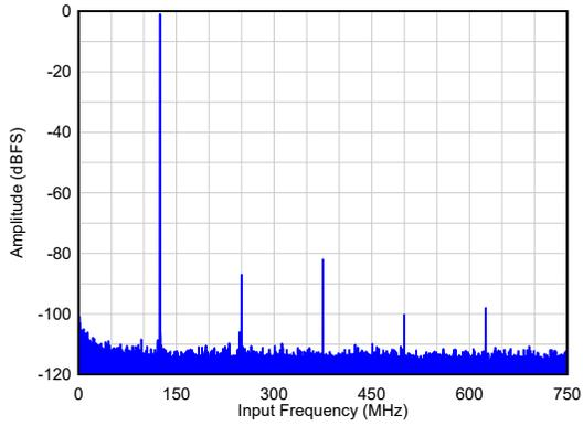
$F_{IN} = 125\text{MHz}$ ,  $A_{IN} = -1\text{dBFS}$ ,  $\text{SNR}_{\text{flat}} = 74.8\text{dBFS}$
