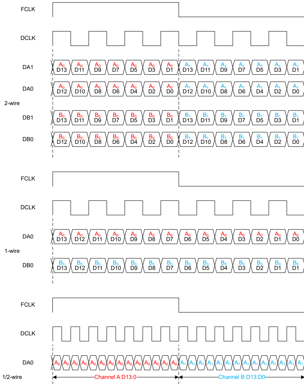
図 7-32. Output Data Format in Real Decimation (14-bit Output Resolution)
