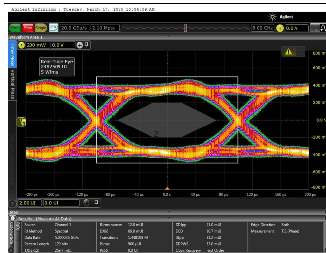
Figure 78. Eye Diagram at 5-Gbps Bit Rate with Default Output Swing
