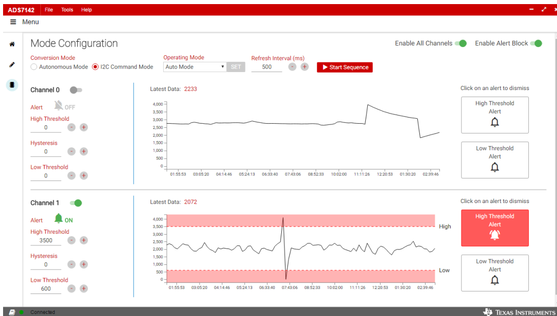
121. Alert Output from ADS7142 with PIR Sensor
