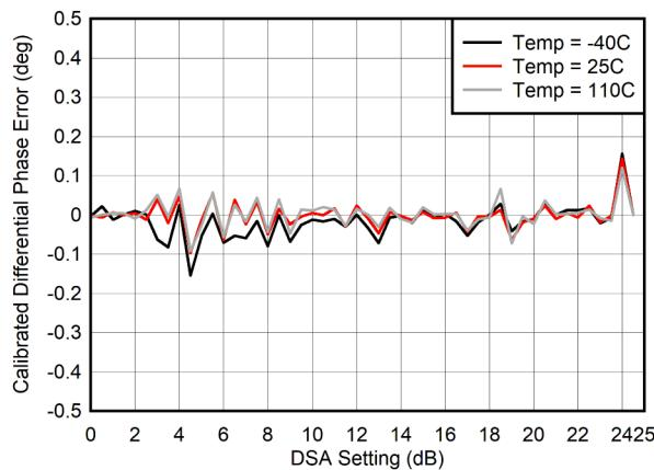
$$\text{微分位相誤差} = \text{Phase}_{\text{IN}}(\text{DSA 設定} - 1) - \text{Phase}_{\text{IN}}(\text{DSA 設定})$$
