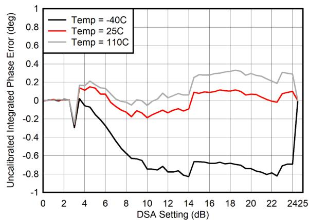
$$\text{積分位相誤差} = \text{Phase}(\text{DSA 設定}) - \text{Phase}(\text{DSA 設定} = 0)$$
