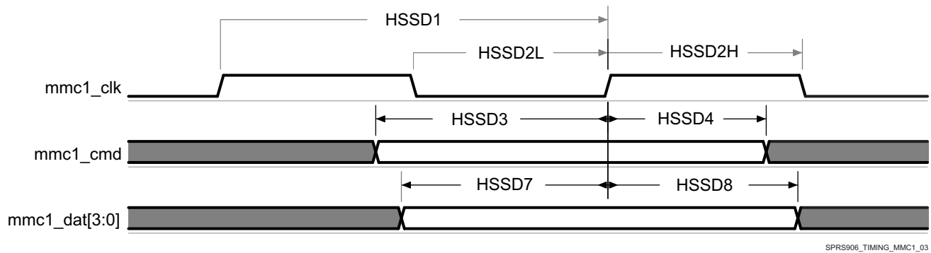
图 5-75. MMC/SD/SDIO in - High Speed - Receiver Mode
