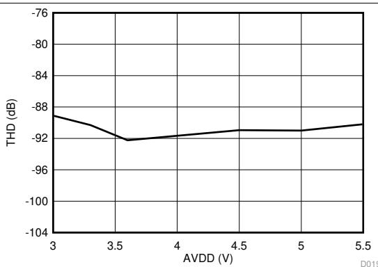
**Figure 24. Total Harmonic Distortion vs High-Side Supply Voltage**
