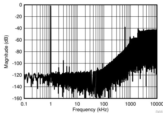
sinc<sup>3</sup> filter, OSR = 1,  $f_{\text{CLKIN}} = 20 \text{ MHz}$ ,  $f_{\text{IN}} = 1 \text{ kHz}$
