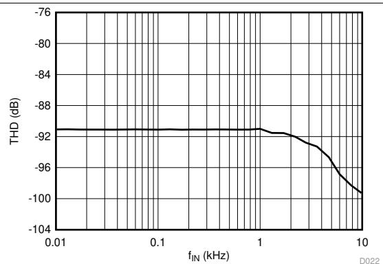
**Figure 27. Total Harmonic Distortion vs Input Signal Frequency**
