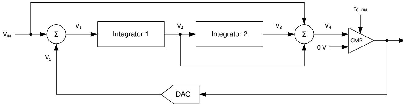
**Figure 42. Block Diagram of a Second-Order Modulator**
