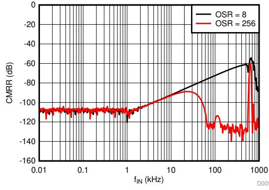
**Figure 17. Common-Mode Rejection Ratio vs Input Signal Frequency**
