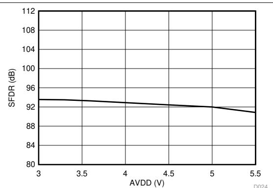
**Figure 29. Spurious-Free Dynamic Range vs High-Side Supply Voltage**
