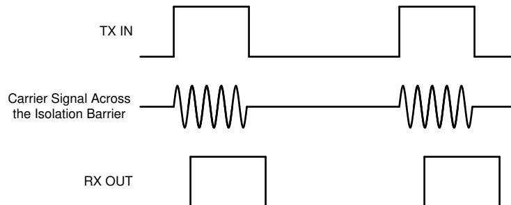
**Figure 44. OOK-Based Modulation Scheme**
