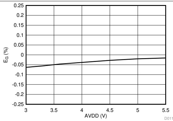
**Figure 14. Gain Error vs High-Side Supply Voltage**
