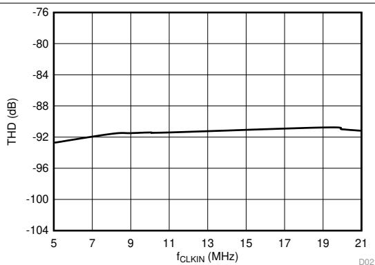
**Figure 26. Total Harmonic Distortion vs Clock Frequency**
