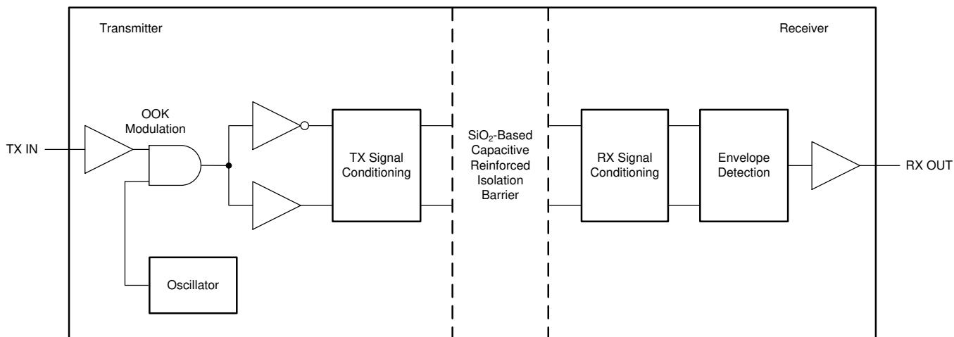
**Figure 43. Block Diagram of an Isolation Channel**
