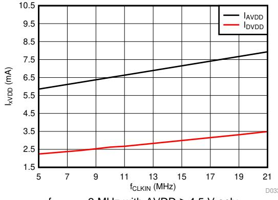
Figure 38. Supply Current vs Clock Frequency
