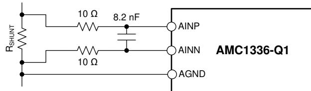
**Figure 52. Differential Input Filter**
