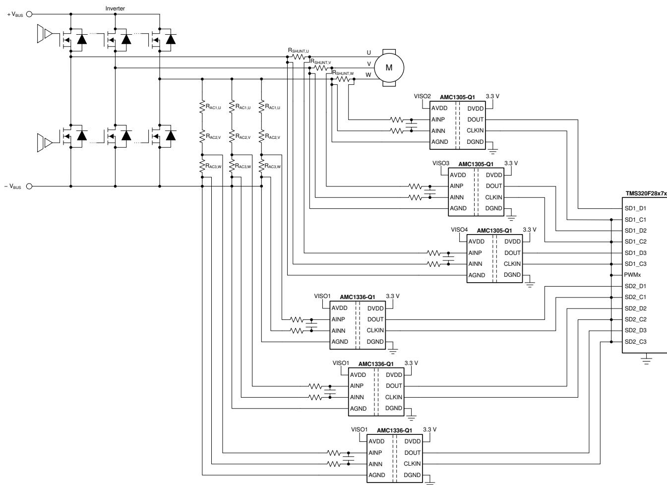
**Figure 50. The AMC1336-Q1 in a Frequency Inverter Application**
