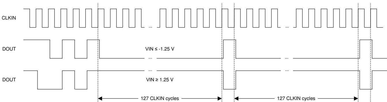
**Figure 48. Out-of-Range Output of the AMC1336-Q1**
