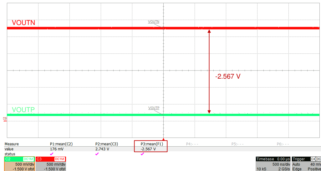
Figure 7-4. Typical Fail-Safe Output of the AMC3311
