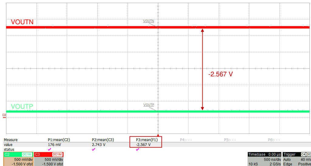
Figure 7-4. Typical Fail-Safe Output of the AMC3311-Q1
