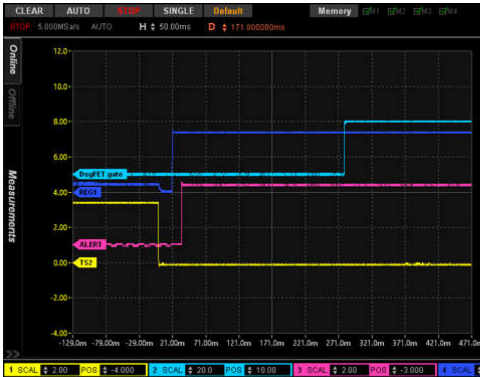
図 8-6. Startup Sequence Using [FASTADC] = 1, with the [INITCOMP] Flag Displayed on the ALERT Pin
