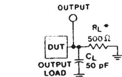
\*FOR AC SERIES ONLY: WHEN  $V_{CC} = 1.5$  V,  $R_L = 1$  k $\Omega$
