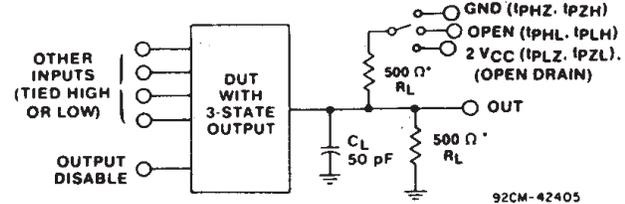
\*FOR AC SERIES ONLY: WHEN  $V_{CC} = 1.5$  V,  $R_L = 1$  k $\Omega$
