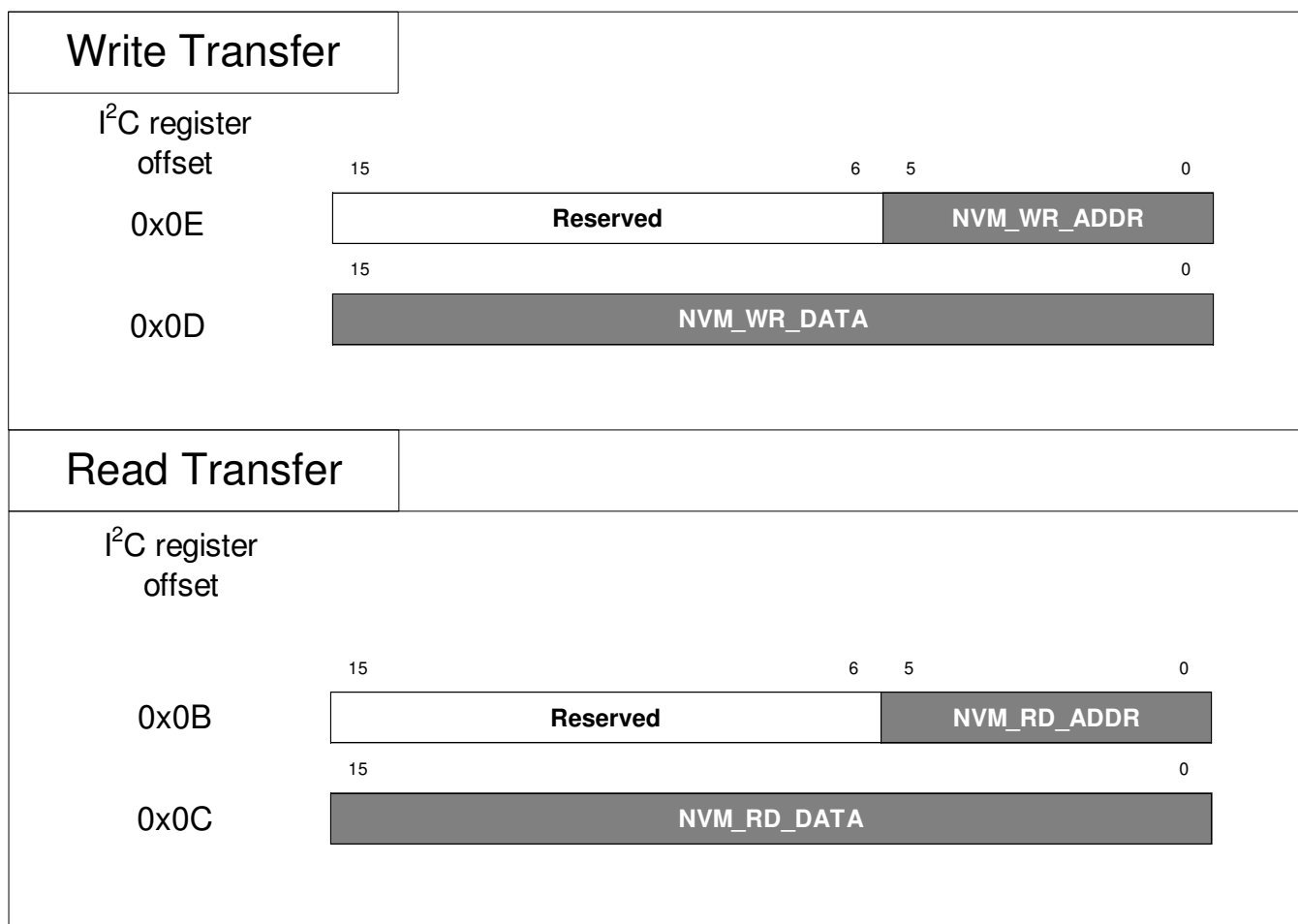
Figure 34. EEPROM Direct Access Using I 2 C
