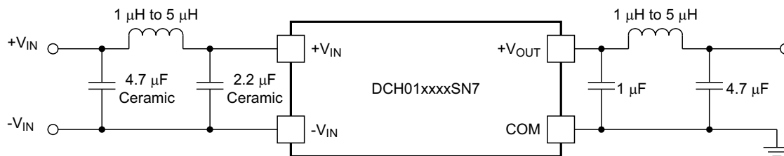
Figure 22. DCH01 Series \pi Filter
