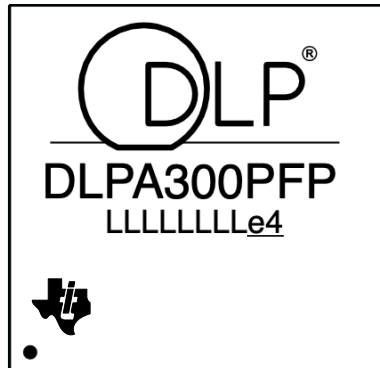
図 11-1. Device Marking (Device Top View)
