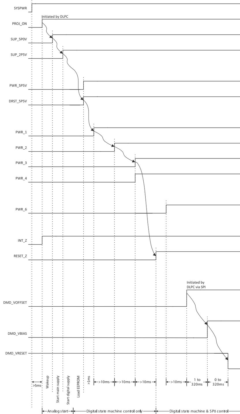
1. Arrows indicate the sequence of events automatically controlled by the digital state machine. Other events are initiated under SPI control.
