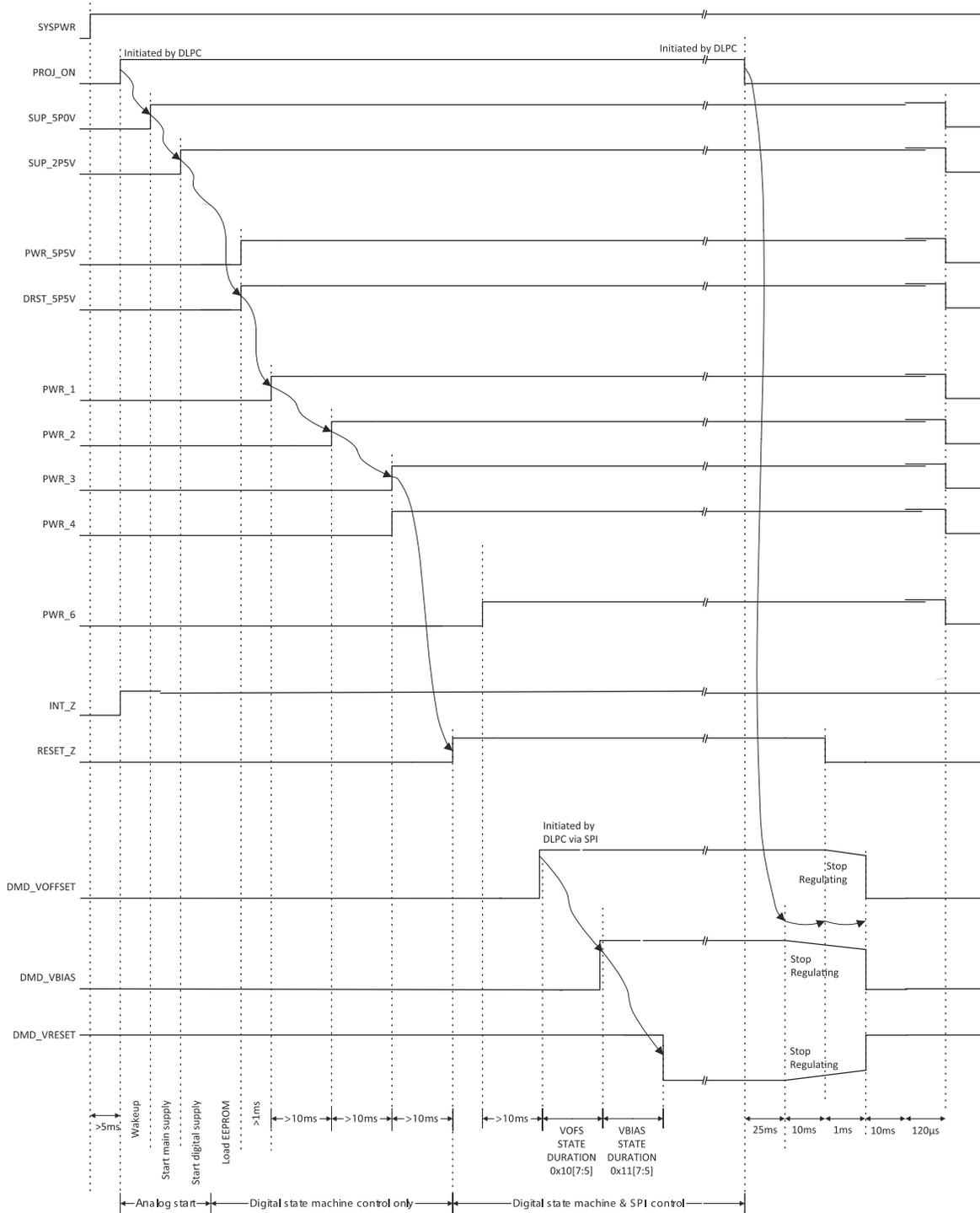
1. Arrows indicate the sequence of events automatically controlled by the digital state machine. Other events are initiated under SPI control.
