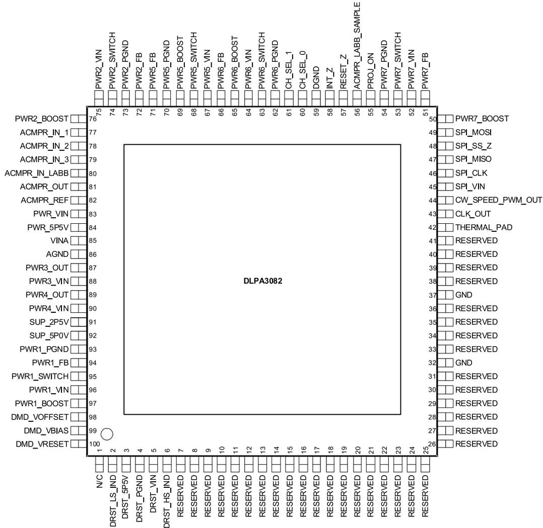
図 4-1. PFD Package 100-Pin HTQFP Top View
