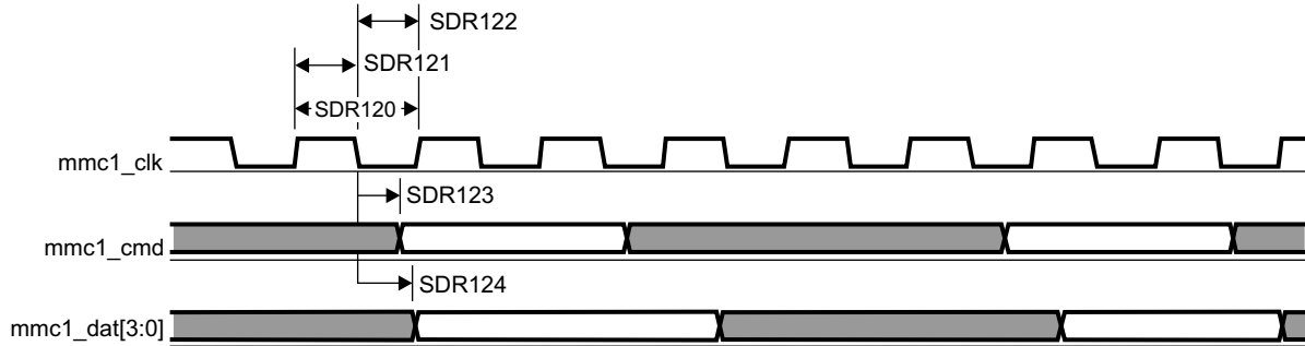
图 7-67. MMC/SD/SDIO in - High Speed SDR12 - Transmitter Mode
