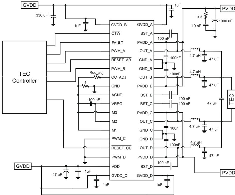
図 7-10. Application Diagram Example for TEC Driver Schematic
