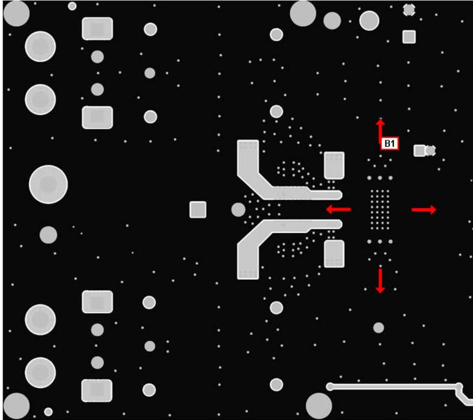
B1: Do not block the heat transfer path at bottom side. Clear as much space as possible for better heat spreading.
