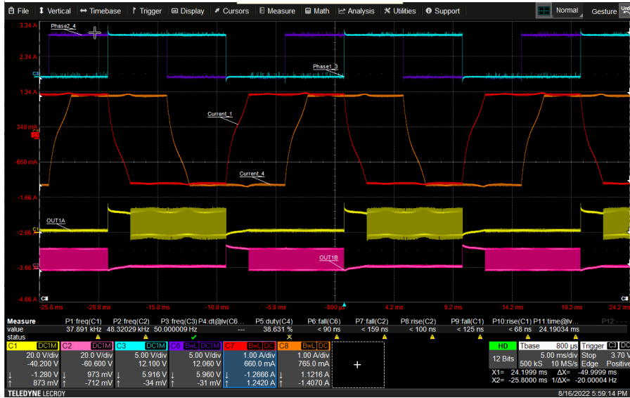
8-2. Driving two stepper motors in full-step
