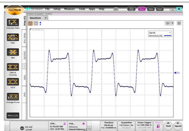
☒ 9-6. DS250DF230 FIR Transmit Equalization While Operating at 25.78125 Gbps
