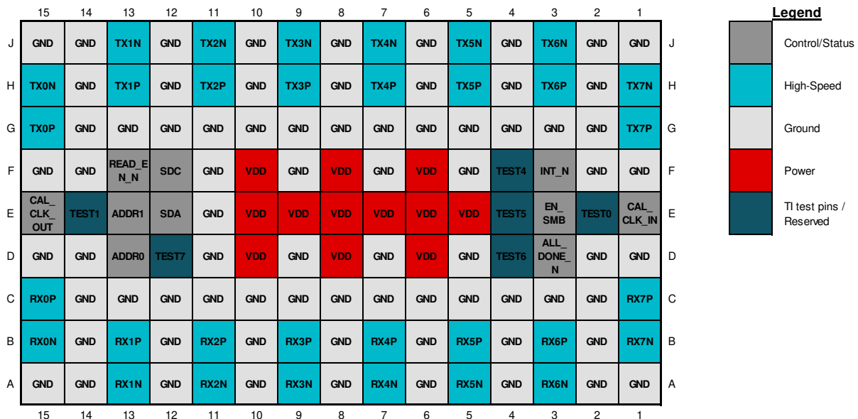
図 4-1. 135-Pin fcBGA, 0.8mm BGA Pin Pitch (Top View)
