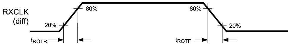
FIGURE 2. LVDS Output Transition Time
