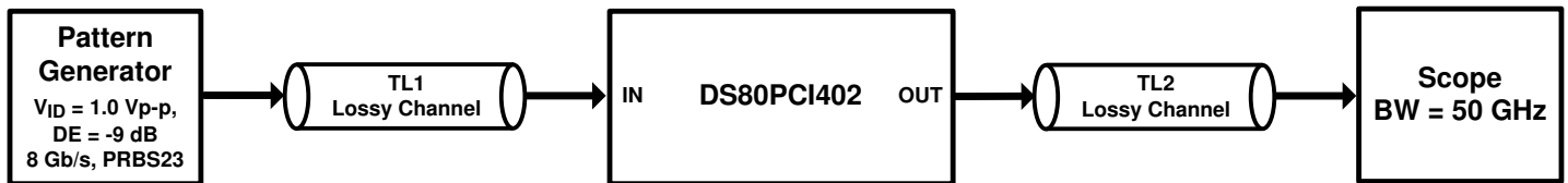
图 9-2. Test Setup Connections Diagram
