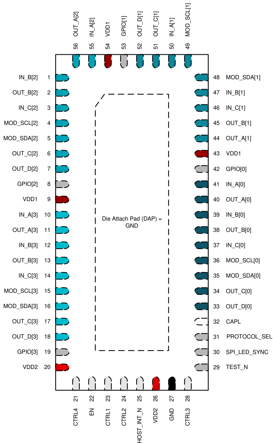
图 6-1. RHU Package 56-Pin WQFN Top View
