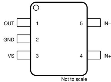
**图 5-1. INA290: DCK Package 5-Pin SC-70 Top View**
