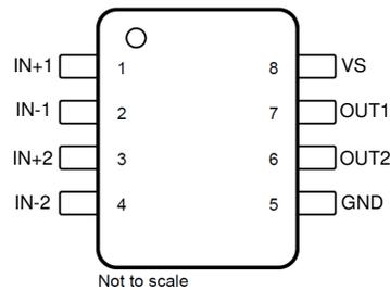
**图 5-2. INA2290: DGK Package 8-Pin VSSOP Top View**
