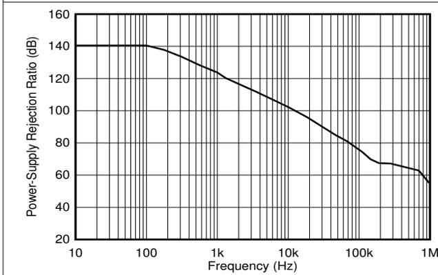
6-13. Power-Supply Rejection Ratio vs. Frequency
