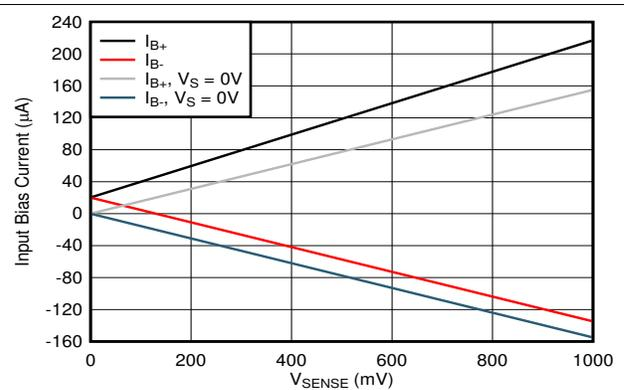
6-16. Input Bias Current vs.  $V_{\text{SENSE}}$ , A1 Devices
