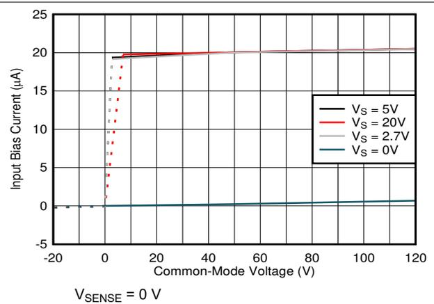
6-14. Input Bias Current vs. Common-Mode Voltage
