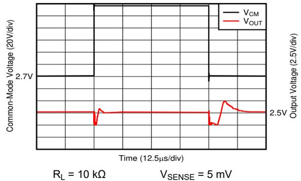
**6-40. Common-Mode Voltage Fast Transient Pulse, A5 Devices**
