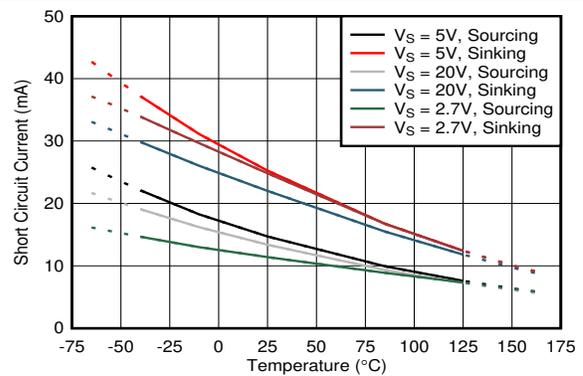
6-22. Short-Circuit Current vs. Temperature
