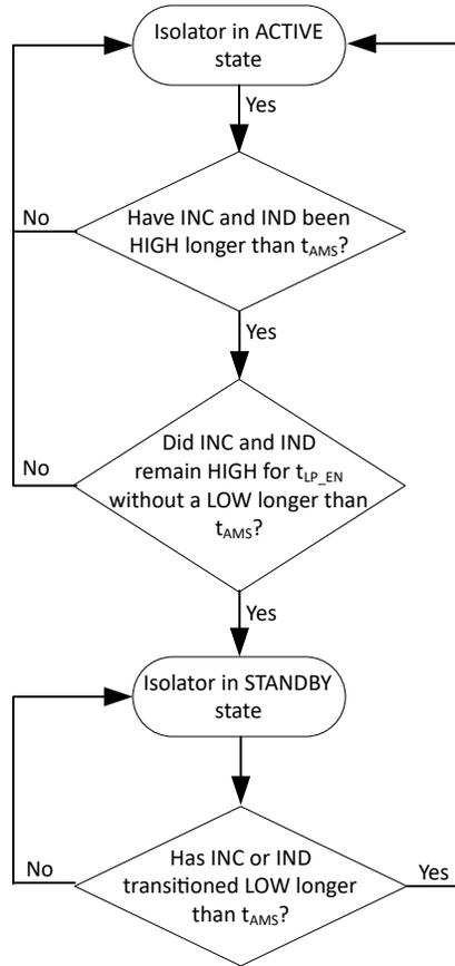
图 7-2. Low-Speed Control Channel Automatic Enable State Changes Flowchart
