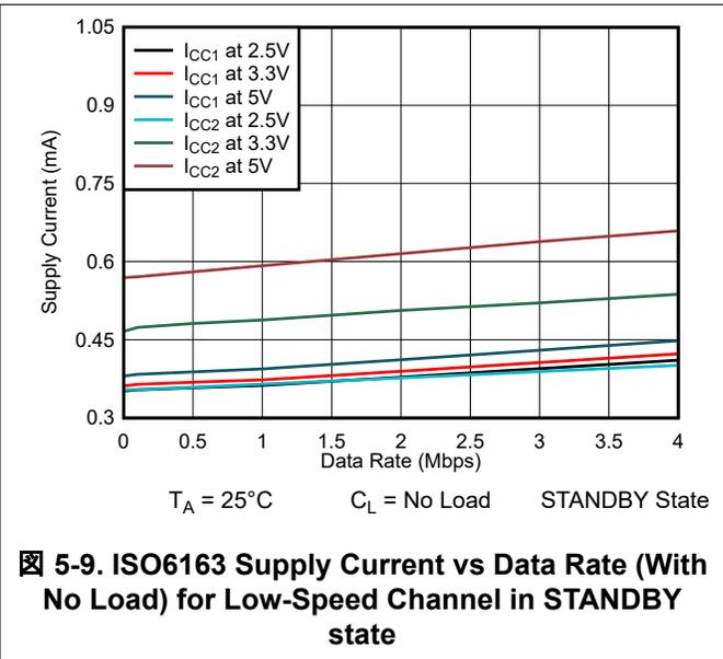
5.19.4 Typical Characteristics: Low-Speed Control Channels (ACTIVE and STANDBY States)
