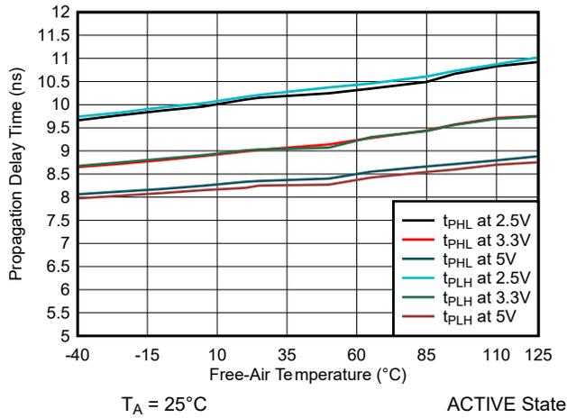
5-5. ISO6163 Propagation Delay Time vs Free-Air Temperature for High-Speed Channel
