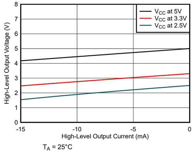
图 5-11. ISO6163 High-Level Output Voltage vs High-level Output Current for Low-Speed Control Channel
