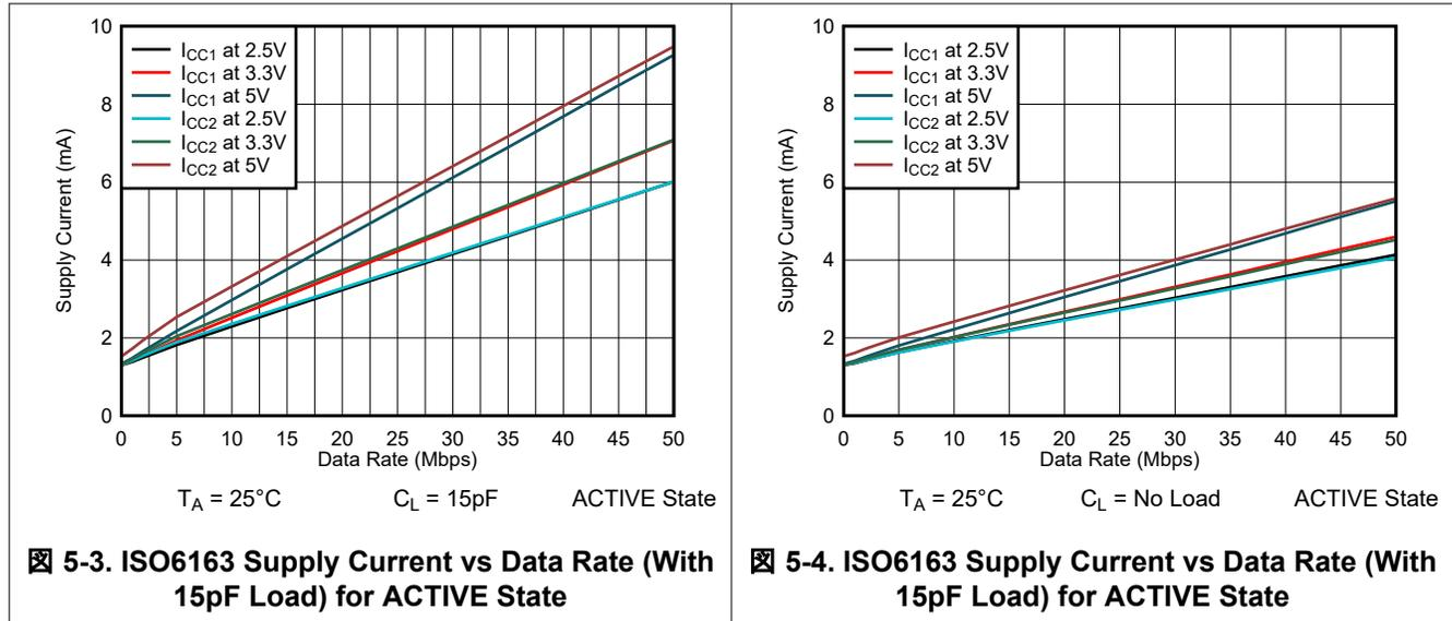
5.19.2 Typical Characteristics: High-Speed Channels (ACTIVE state)
