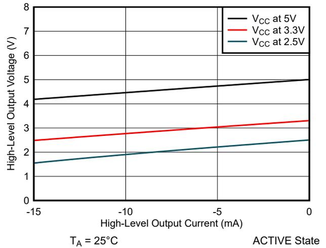
5-6. ISO6163 High-Level Output Voltage vs High-level Output Current for High-Speed Channel
