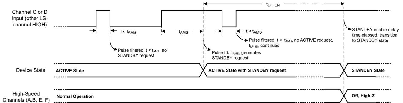
图 7-3. Low-Speed Control Channel Automatic Enable, Case 1 (ACTIVE to STANDBY Example)
