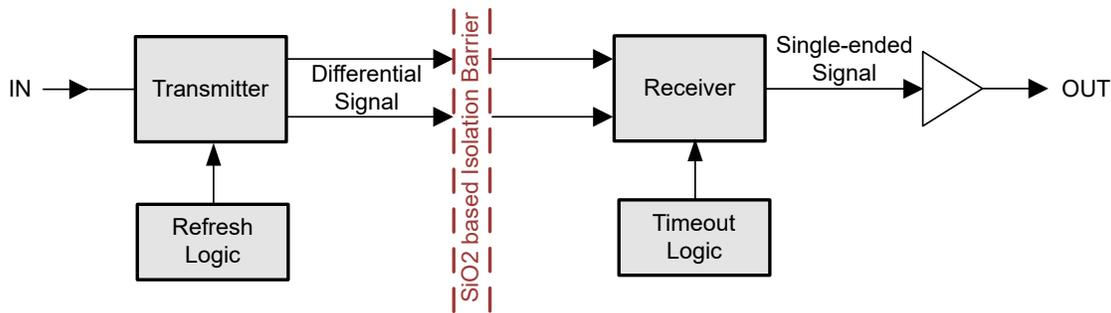
図 7-1. Conceptual Block Diagram of a Digital Isolator
