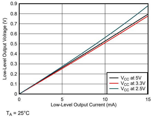
图 5-12. ISO6163 Low-Level Output Voltage vs Low-Level Output Current for Low-Speed Control Channel
