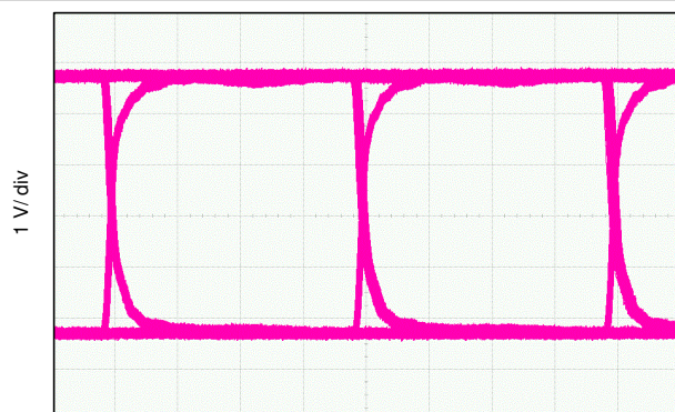
10-3. Eye Diagram at 50 Mbps PRBS 2^{16} - 1 , 5 V and 25°C
