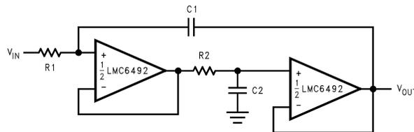
$$R1 = R2, C1 = C2; f = \frac{1}{2\pi R1 C1}; \text{Damping Factor} = \frac{1}{2} \sqrt{\frac{C2}{C1}} \sqrt{\frac{R2}{R1}}$$
