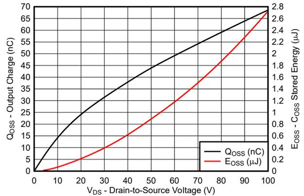
Figure 5-4. Typical Output Charge and  $C_{OSS}$  Stored Energy
