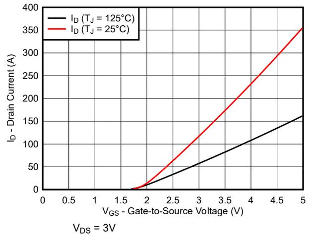
Figure 5-2. Typical Transfer Characteristics
