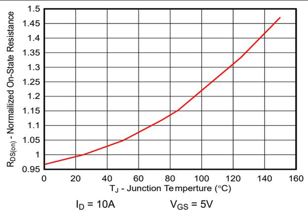
Figure 5-6. Normalized On-State Resistance vs Temperature
