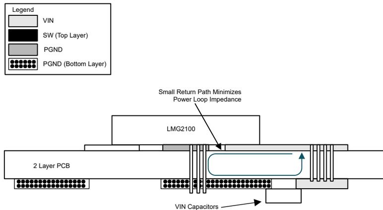
**8-10. Two-Layer Board Cross Section With Return Path**
