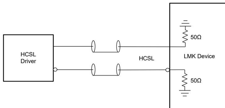
図 8-14. HCSSL (Load Terminated) to Reference (INx)
