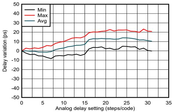
**6-22. SYSREF/1PPS Delay Linearity vs. Analog Delay Code 4**
