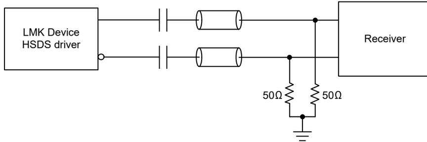
図 8-29. AC-Coupled HSDS Output Termination Method 2
