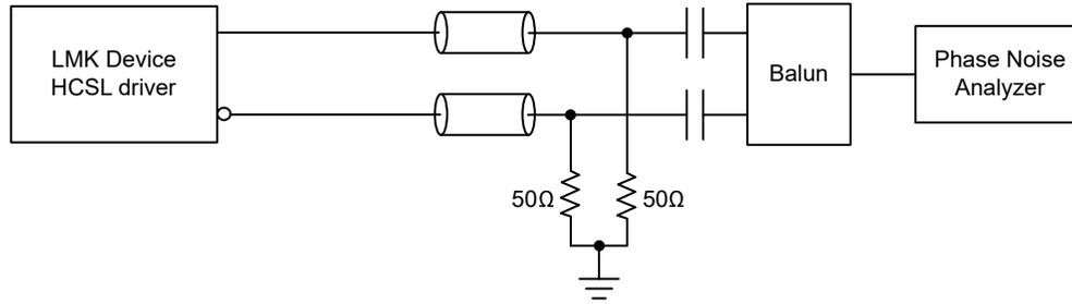
図 7-8. HCSL Output Phase Domain Test Configuration
