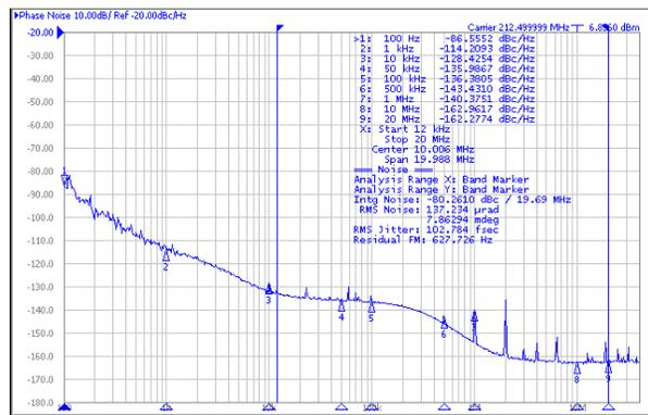
Jitter = 103fs RMS (12kHz to 20MHz)
