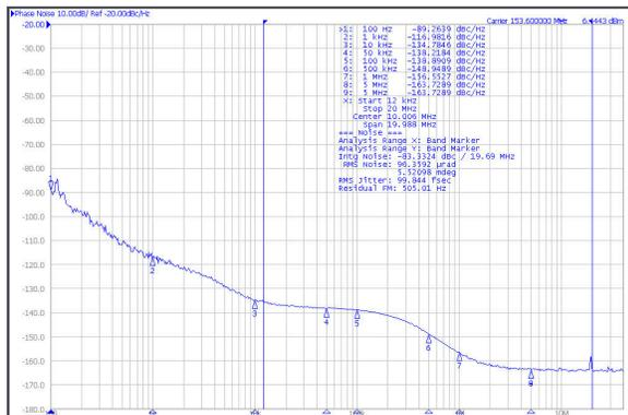
Jitter = 100fs RMS (12kHz to 20MHz)
