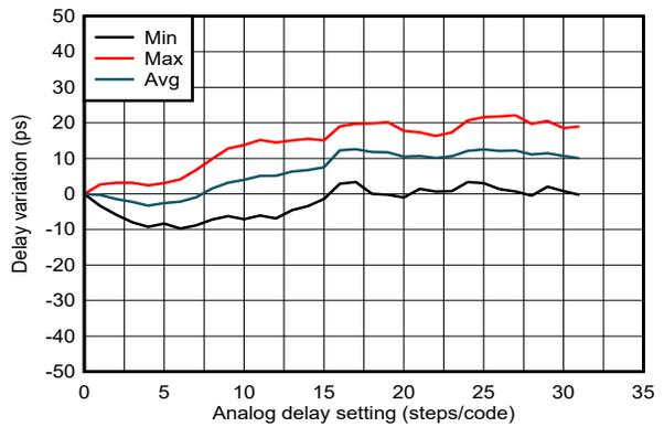
**6-23. SYSREF/1PPS Delay Linearity vs. Analog Delay Code 5**
