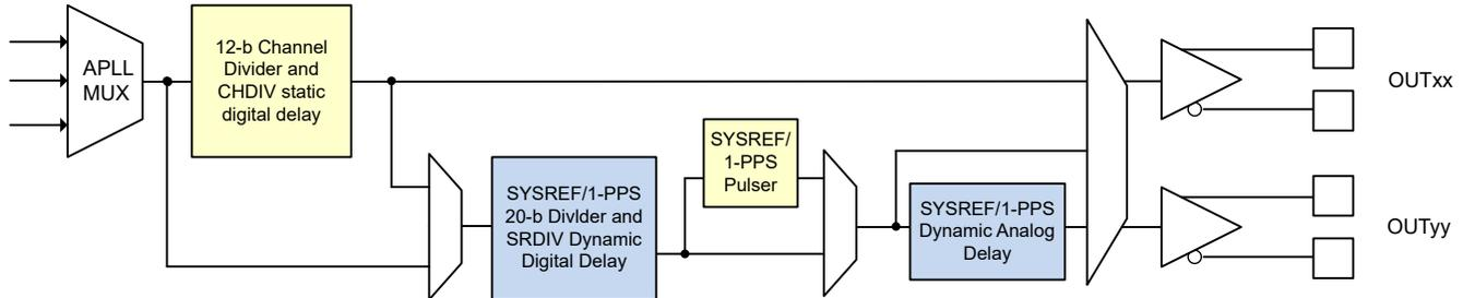
図 8-25. Programmable Static and Dynamic Output Delay
