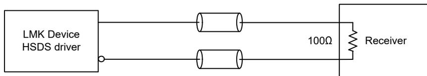
図 8-27. DC-Coupled HSDS/LVDS Output Termination
