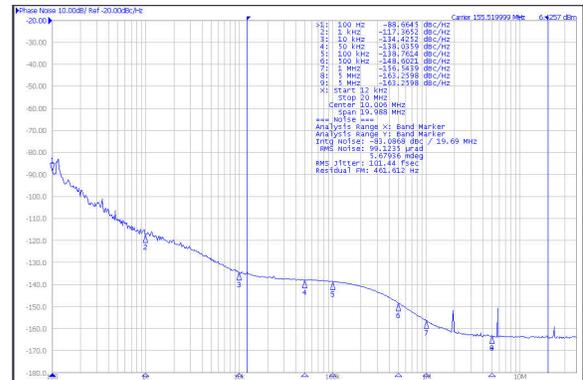
Jitter = 101fs RMS (12kHz to 20MHz)
