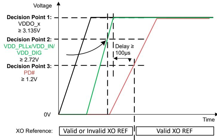
Figure 9-2. Recommendation for Power Up From Split-Supply Rails
