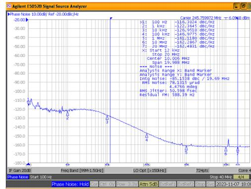
Jitter = 51fs RMS (12kHz to 20MHz)
