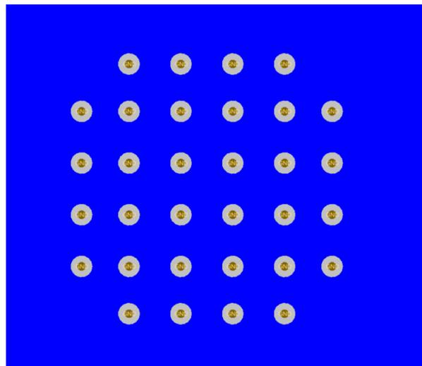
図 9-6. PCB Layout Example for LMK5C33414A, Bottom Layer
