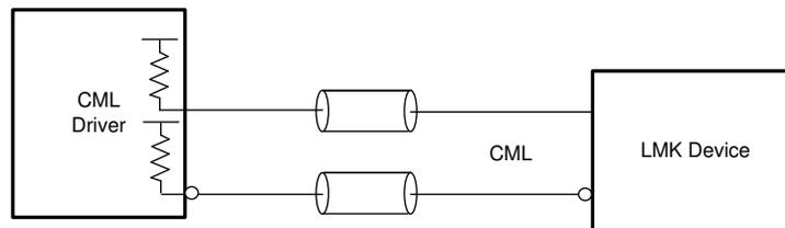
図 8-13. DC-Coupled CML (Source Terminated) to Reference (INx)
