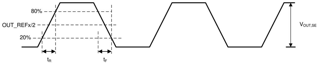
図 6-6. Single-Ended Output Voltage and Rise/Fall Time
