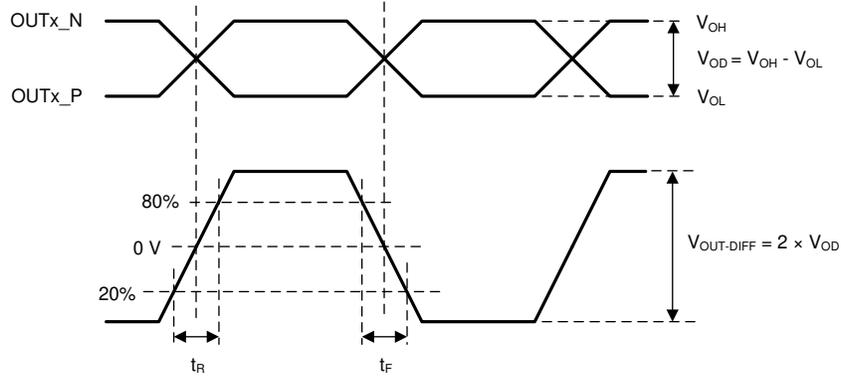
図 6-5. Differential Output Voltage and Rise/Fall Time
