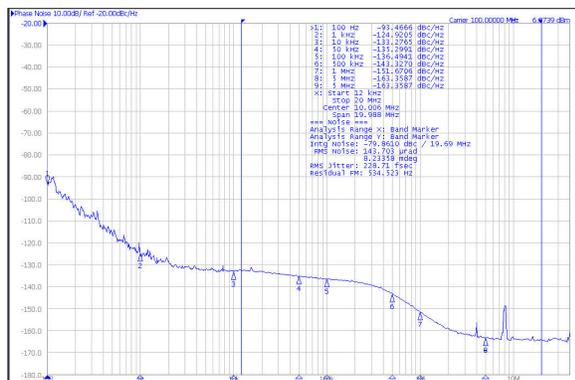
Jitter = 230fs RMS (12kHz to 20MHz)
