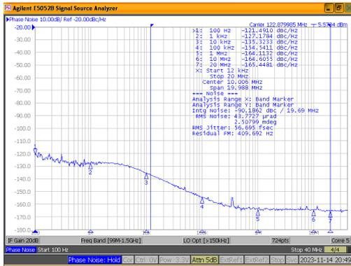
Jitter = 57fs RMS (12kHz to 20MHz)
