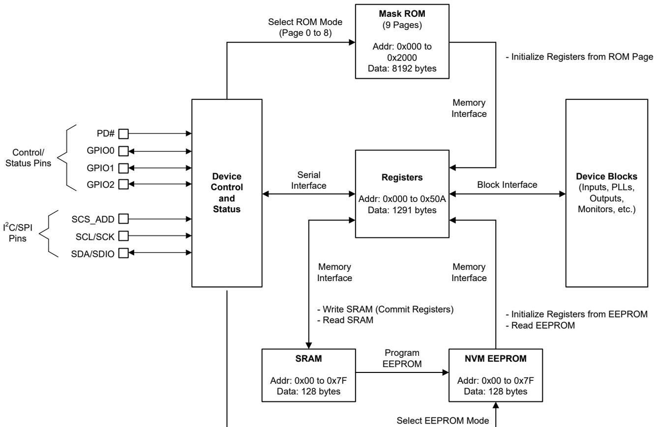
図 8-43. Device Control, Register, and Memory Interfaces
