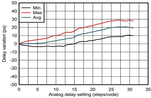
**6-20. SYSREF/1PPS Delay Linearity vs. Analog Delay Code 2**
