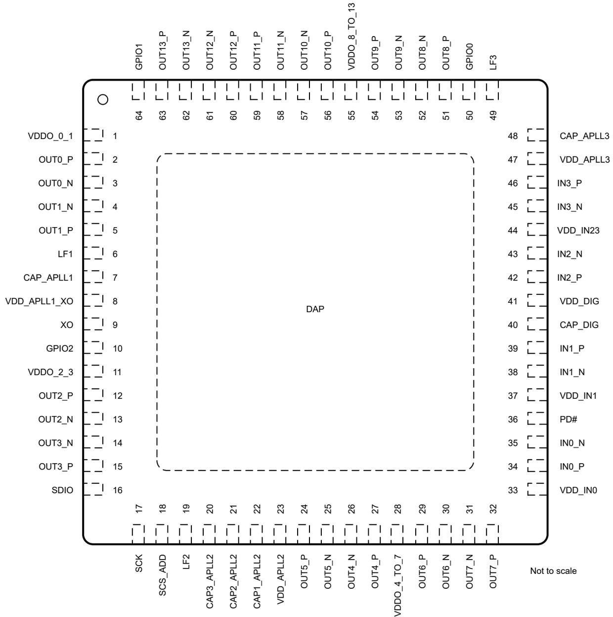
図 5-1. LMK5C33414A RGC Package 64-Pin VQFN Top View
