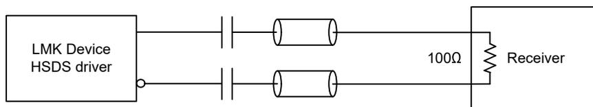
図 8-28. AC-Coupled HSDS Output Termination Method 1
