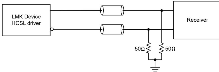
図 8-30. DC-Coupled HCSL Output Termination
