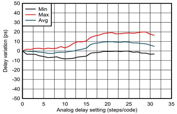
**6-21. SYSREF/1PPS Delay Linearity vs. Analog Delay Code 3**
