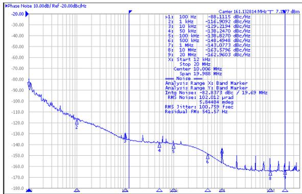
Jitter = 101fs RMS (12kHz to 20MHz)
