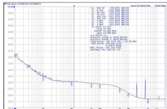
Jitter = 345fs RMS (12kHz to 20MHz)
