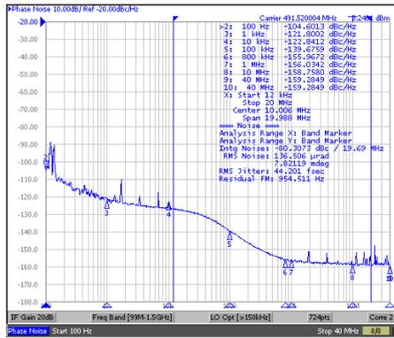
Jitter = 44fs RMS (12kHz to 20MHz)
