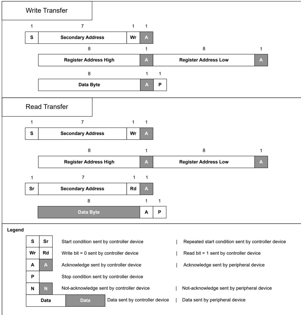
図 8-45. I<sup>2</sup>C Byte Write and Read Transfers
