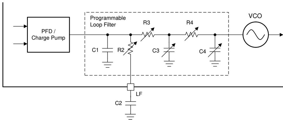
図 8-24. Loop Filter Structure of Each APLL
