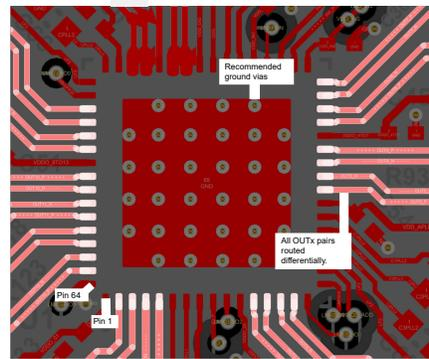
図 9-5. PCB Layout Example for LMK5C33414A, Top Layer
