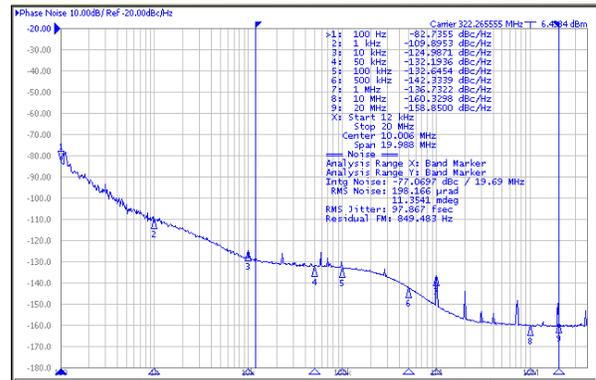
Jitter = 98fs RMS (12kHz to 20MHz)
