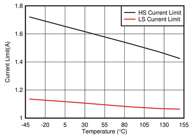
7-10. HS and LS Current Limit versus Temperature
