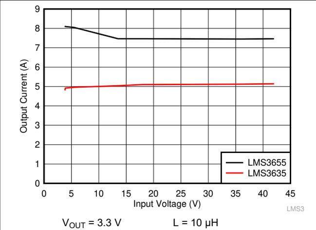
**9-26. Output Current Level for Overcurrent Protection Trip**
