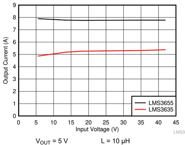
**9-13. Output Current Level Limit Before Overcurrent Protection**
