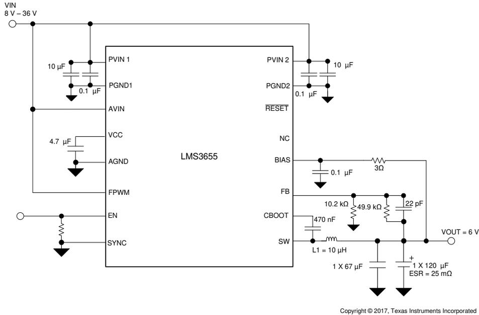
**图 9-30. 6-V Output Power Supply**
