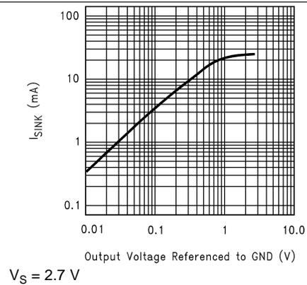
Figure 6. Sinking Current vs. Output Voltage
