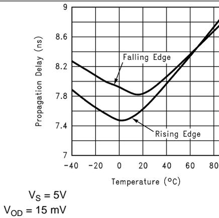
Figure 9. Propagation Delay vs. Temperature
