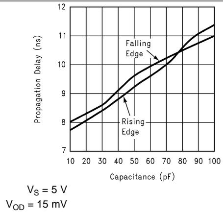
Figure 10. Propagation Delay vs. Capacitive Load
