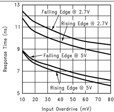
Figure 11. Propagation Delay vs. Input Overdrive
