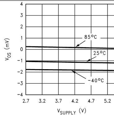
Figure 2.  $V_{OS}$  vs. Supply Voltage
