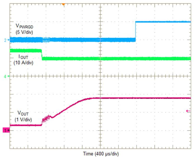
Figure 33. Removal Of Overcurrent (Cycle-By-Cycle)
