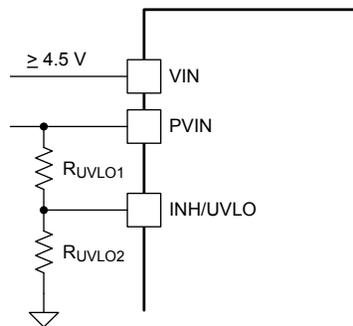
**Figure 41. Adjustable PVIN Undervoltage Lockout, (VIN  $\geq 4.5$  V)**
