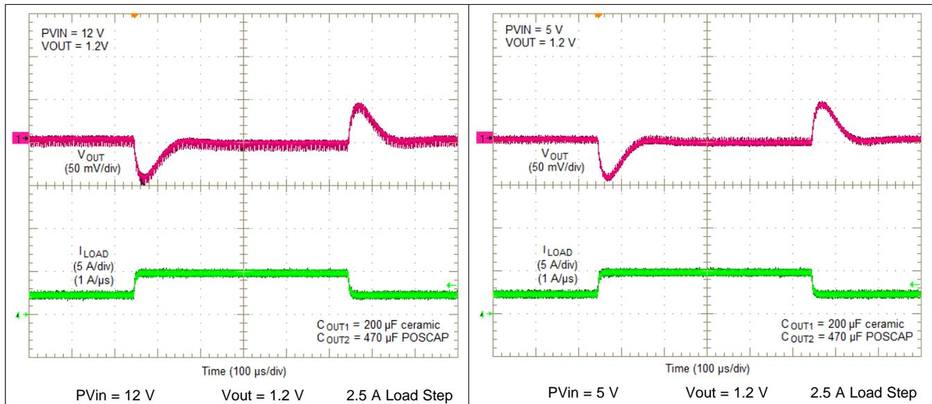
**Figure 19. Transient Response (12 V to 1.2 V)**
