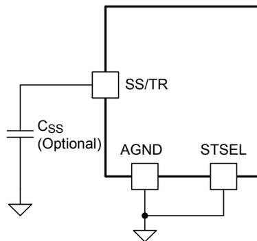
**Figure 29. Slow-Start Capacitor ( $C_{SS}$ ) And STSEL Connection**
