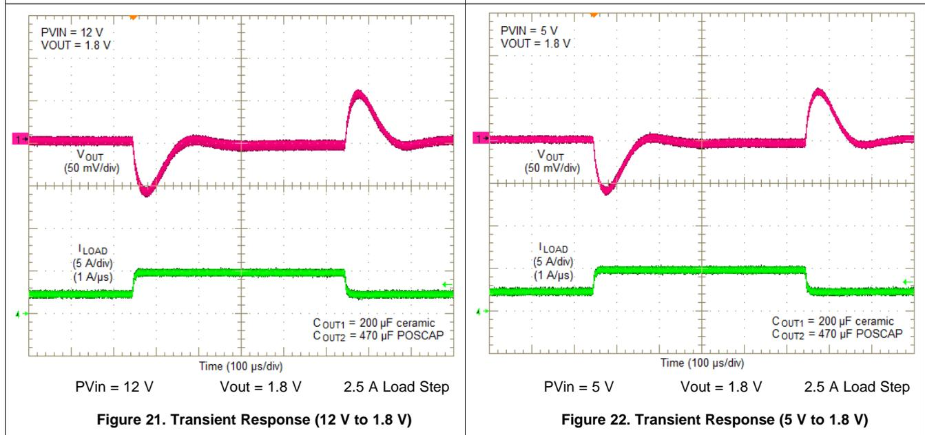
**Figure 21. Transient Response (12 V to 1.8 V)**
