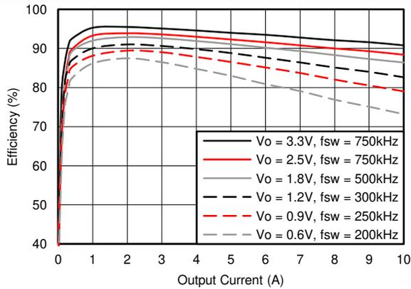
Figure 7. Efficiency versus Output Current
