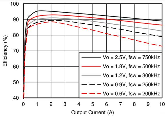
Figure 12. Efficiency versus Output Current
