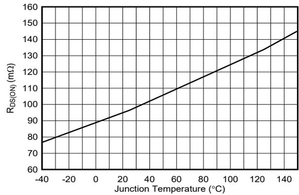
7-2.  $R_{DS(ON)}$  (high and low side combined) for MOSFETs over temperature
