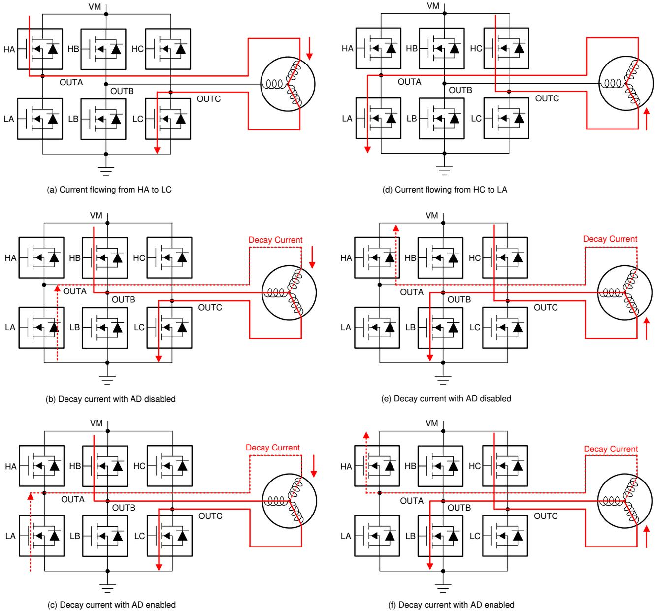
**Figure 8-38. Active Demagnetization in BLDC Motor Commutation**
