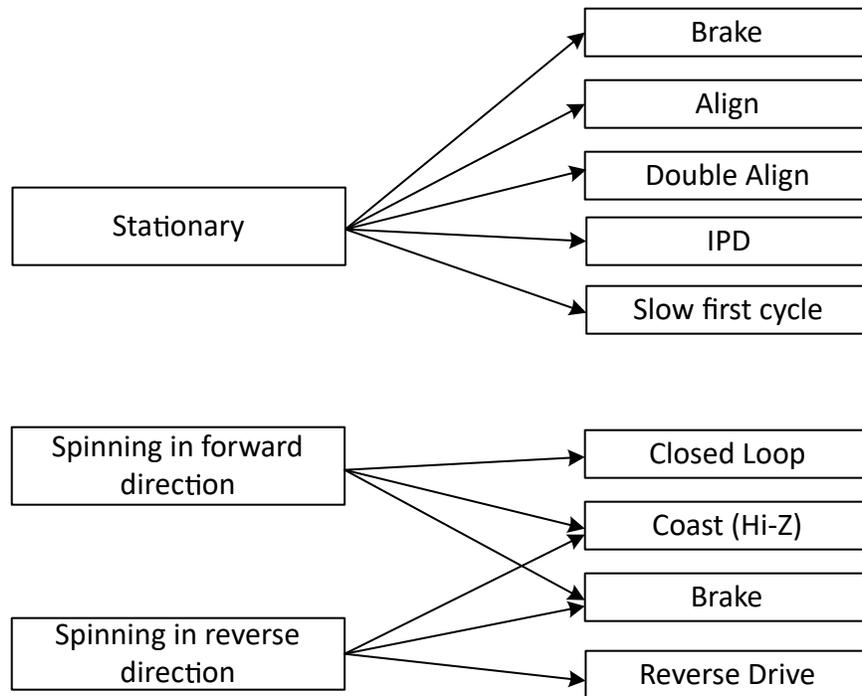
**8-18. Starting the motor under different initial conditions**
