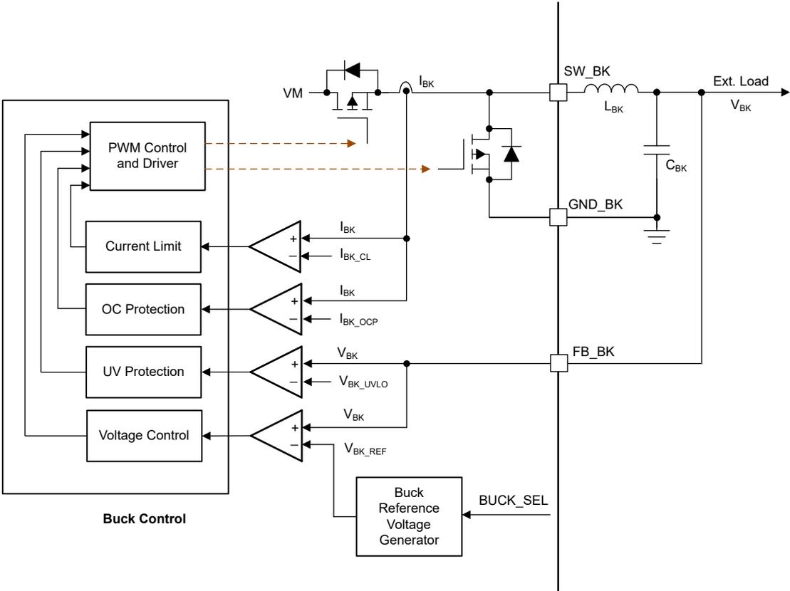
shows the architecture of the buck and various control/protection loops.
