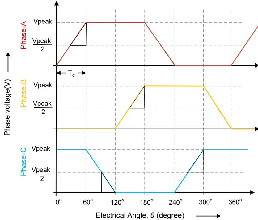
**图 8-35. Back-EMF integration using floating phase voltage**
