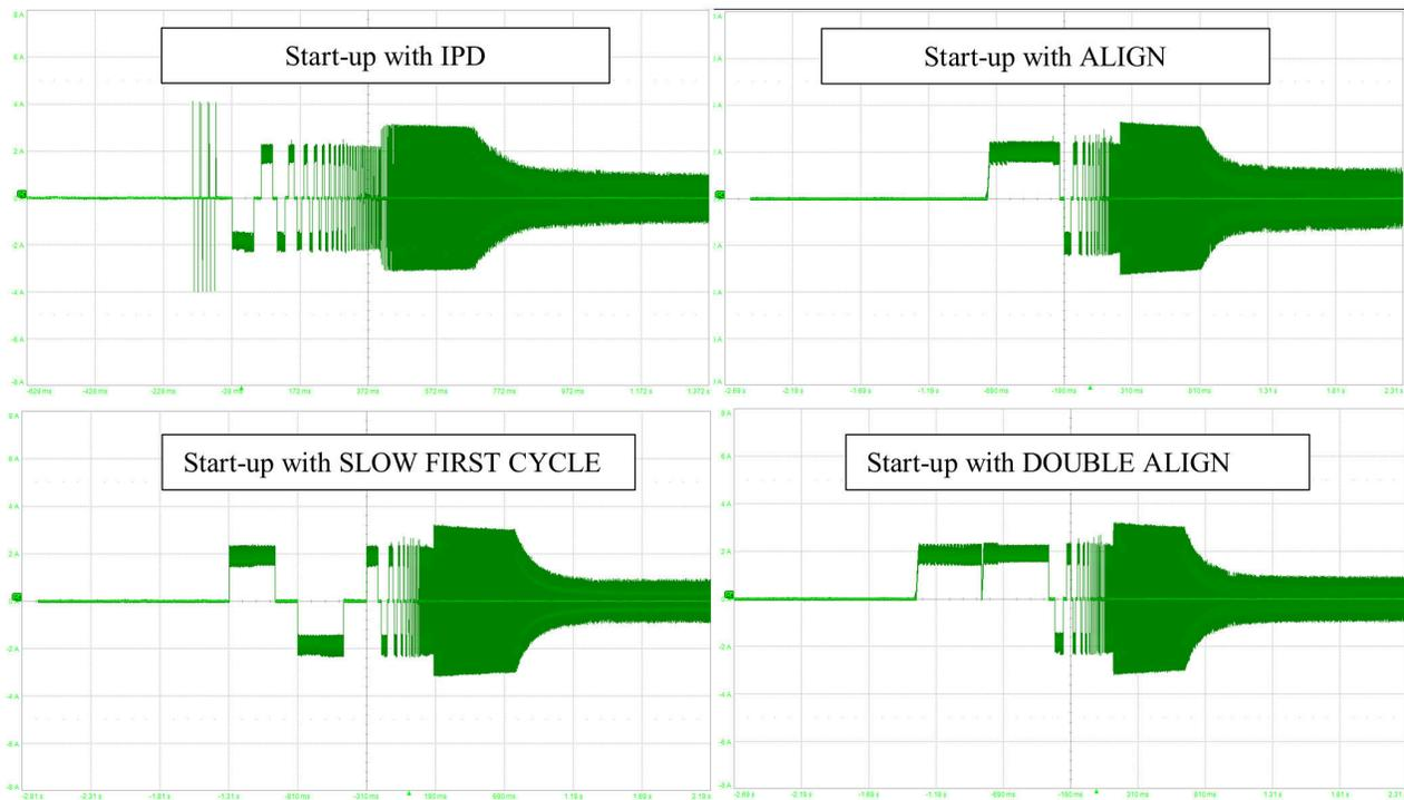
☒ 9-2. Motor phase current waveforms of all startup methods
