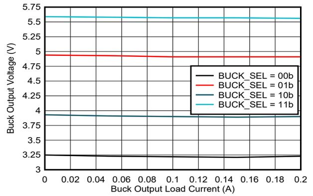
7-4. Buck regulator output voltage over load current
