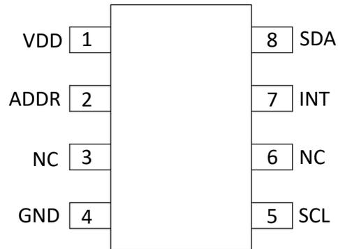
図 4-1. DTS Package, 8-Pin SOT 5X3, Top View
