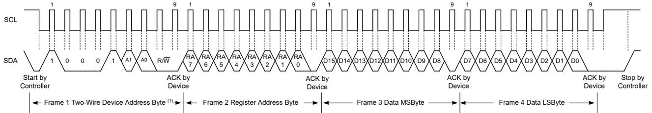
Figure 6-5. I<sup>2</sup>C Write Example
