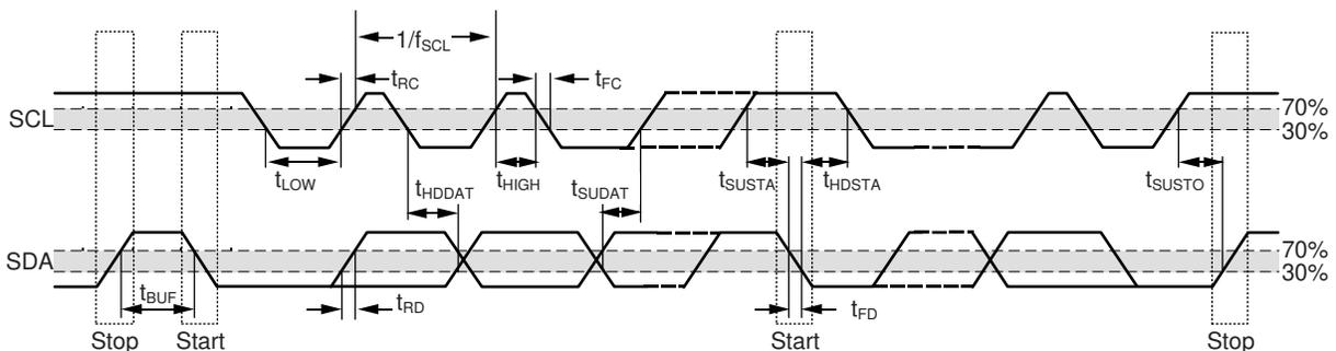
5-1. I<sup>2</sup>C Detailed Timing Diagram
