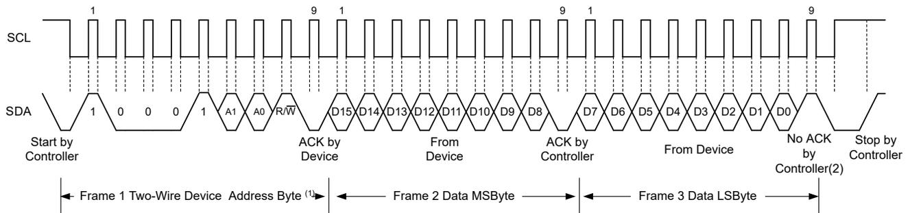
A. An ACK by the controller can also be sent.
