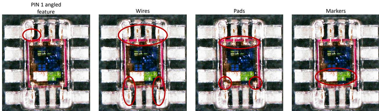
図 8-5. Identification Features for PIN 1 on Package
