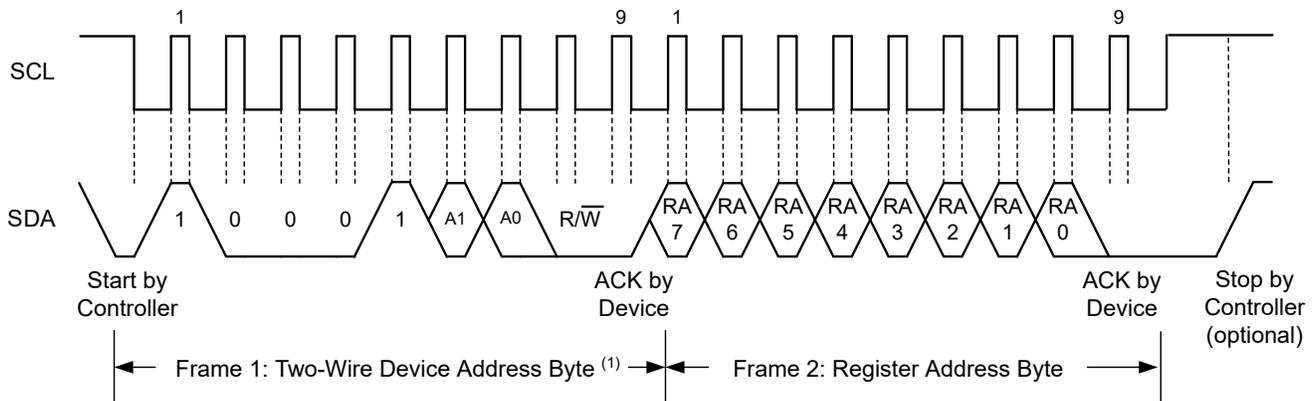
図 6-4. Setting the I<sup>2</sup>C Register Address
