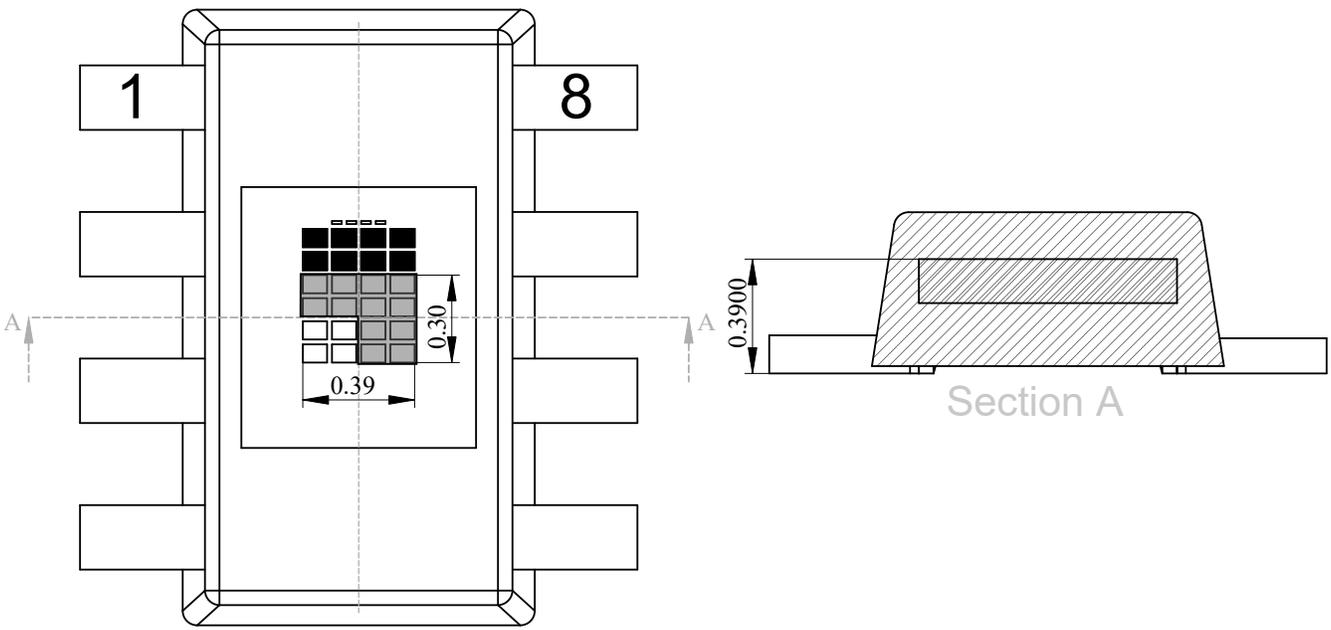
8-2 shows the dimensions of the optical area. The gray area indicates the channel 0 photodiode and the white area indicates the channel 1 photodiode.
