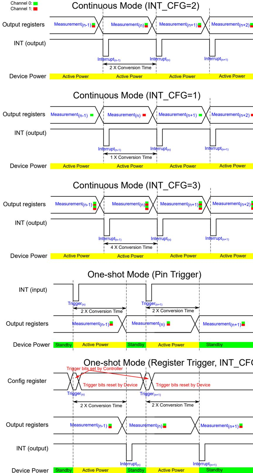
図 6-2. Timing Diagrams for Different Operating Modes
