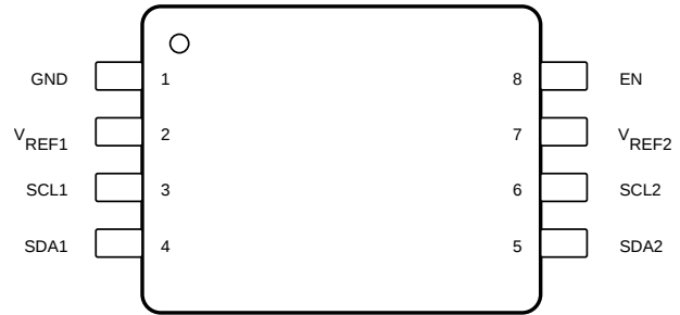
图 5-2. DCU Package 8-Pin VSSOP (Top View)
