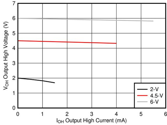
**6-1. Typical output voltage in the high state (V<sub>OH</sub>)**
