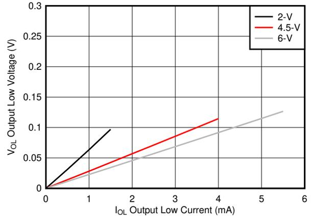
**6-2. Typical output voltage in the low state (V<sub>OL</sub>)**
