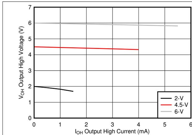
Figure 6-1. Typical output voltage in the high state (V<sub>OH</sub>)
