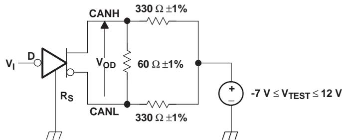
Figure 14. Driver  $V_{OD}$
