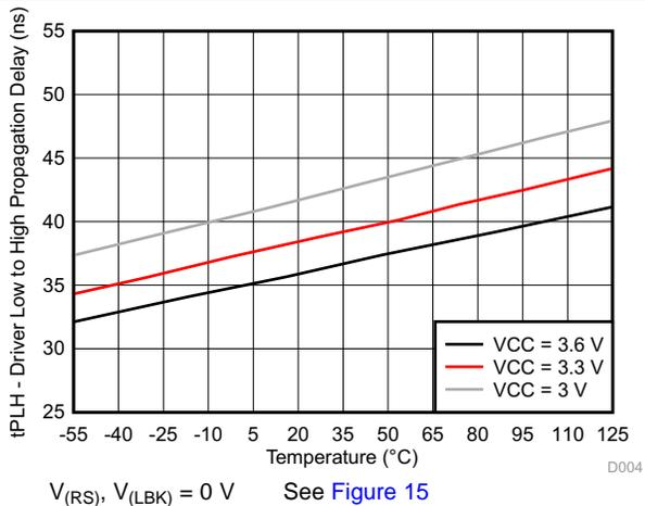
Figure 9. Driver Low-To-High Propagation Delay vs Temperature
