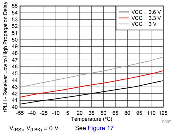
Figure 7. Receiver Low-To-High Propagation Delay vs Temperature
