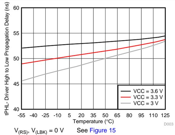
Figure 10. Driver High-To-Low Propagation Delay vs Temperature
