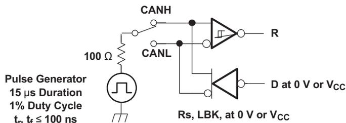
NOTE: This test is conducted to test survivability only. Data stability at the R output is not specified.
