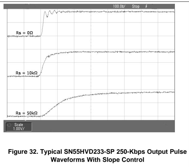
**Figure 32. Typical SN55HVD233-SP 250-Kbps Output Pulse Waveforms With Slope Control**
