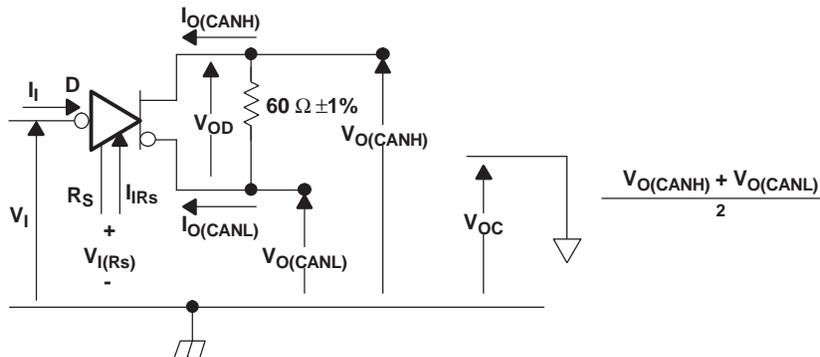
Figure 12. Driver Voltage, Current, and Test Definition
