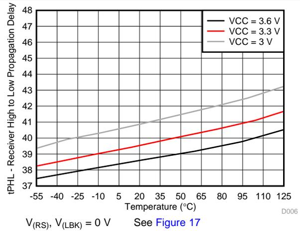
Figure 8. Receiver High-To-Low Propagation Delay vs Temperature
