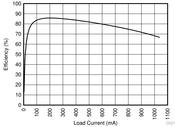
SN6505B + Würth 750316028 V_{CC} = 3.3\text{ V}
