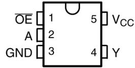
図 5-1. SN74AHC1G125-Q1 DBV Package, 5-Pin SOT-23; DCK Package, 5-Pin SC-70 (Top View)
