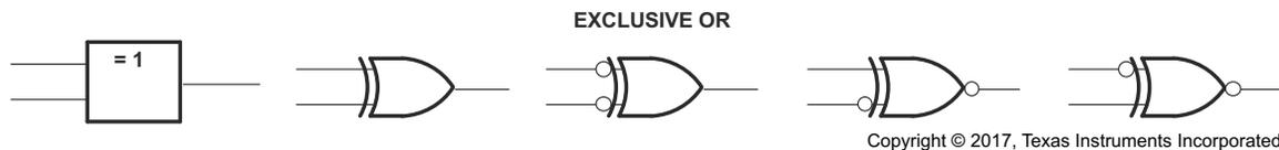
These are five equivalent exclusive-OR symbols valid for an SN74AHC1G86-Q1 gate in positive logic; negation may be shown at any two ports.
