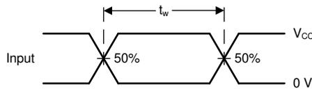
6-2. Voltage Waveforms, Standard CMOS Inputs Pulse Duration
