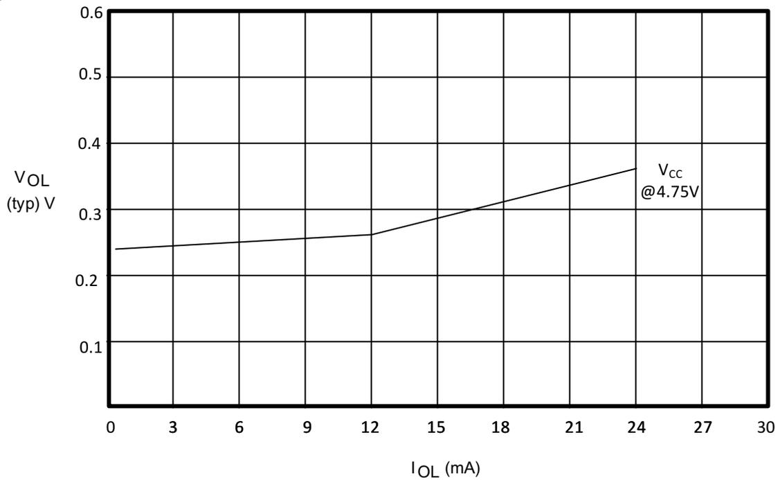
**Figure 3. V<sub>OL</sub> vs I<sub>OL</sub>**
