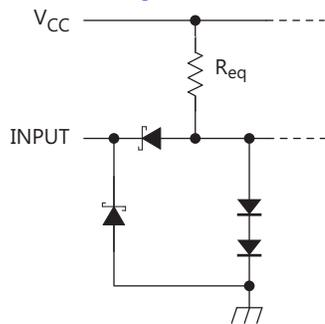
**Figure 7. Equivalent of Each Input**
