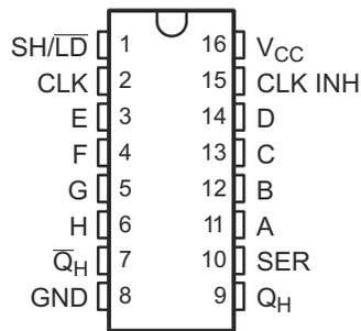
图 5-1. D, DB, DGV, N or PW Package,
