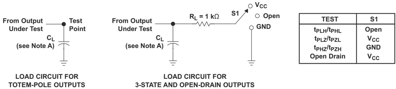
LOAD CIRCUIT FOR TOTEM-POLE OUTPUTS
