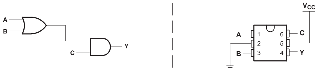
Figure 3. Y = (A + B) \bullet C
