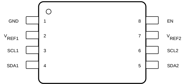
☒ 5-2. DCU Package, 8-Pin VSSOP, Top View
