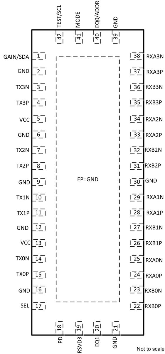
図 4-1. RUA Package, 42-Pin WQFN (Top View)
